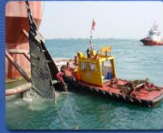
Anchor Recovery For Oil Rig
