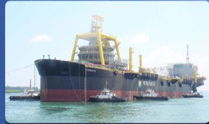
Hooking Up Of Vessel FPSO P53 To Temporary 6pts Mooring System
