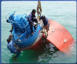
SSE Divers - Cleaning Of Thruster Flange Before Installation
