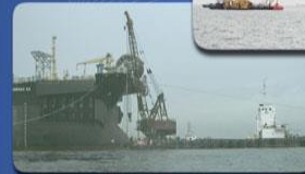
← ↑ Hooking Up Of Vessel "Petrobas 54" To 06 Point Mooring System At Raffles Reserved Anchorage
