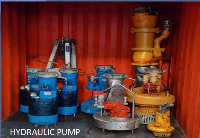
HYDRAULIC CARGO TRANSFER PUMP 66 cu.m per.hr 1,000,000 CST
