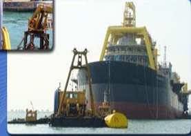
→ Hooking Up Of 6 Point Mooring System For FPSO Vessel - P53
