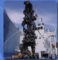
Removing Ropes After Disentangling Anchor From Anchor Chain
