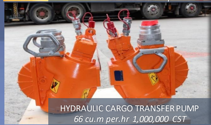
PORTABLE HYDRAULIC SUBMERSIBLE CARGO PUMPS – 150 cu.m per hour
